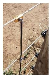
You can now connect your energizer to the Equirope<sup>™</sup>. Run a length of underground wire from the positive terminal on your energizer to the top strand of Equirope<sup>™</sup>. Feed the wire into under the wingnut of the Striker connector and twist around to help lock in place and tighten the wingnut.
